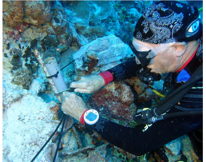
ABOVE | A temperature logger being attached to a stake hammered into the reef. Instruments are commonly located inside a piece of pipe to prevent them being destroyed by grazing fish.
